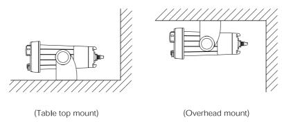
Figure 2-1 Typical Mounting Methods
